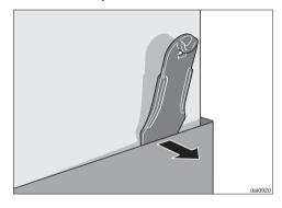
After loosening both of the clamping screws on the chimney, slide the lever between the chimney and the chimney extension and gently apply pressure to ease the chimney from its hooks.
